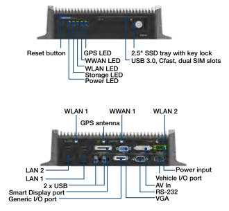
Note: WLAN 1 = WLAN main, WLAN 2 = WLAN auxiliary, WWAN 1 = WWAN main
