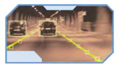
• LDWS: (Lane Departure Warning System) The system is compliant with ISO-17361. LDWS warns the driver when a vehicle is drifting or fails to use the correct turn signal when changing lanes.
