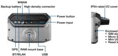
Enclosed I/O SIM slot Micro SD slot Mini USB port Reset key 2 .
