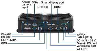
Note: WLAN 1 = WLAN main, WWAN 1 = WWAN main, WWAN 2 = WWAN auxiliary
